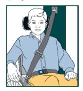
▼ A diagonal shoulder belt should cross the middle of the shoulder and the center of the chest, and should connect to the lap belt near the hip of the wheelchair rider. The upper shoulder-belt anchor point or guide should be anchored above and behind the top of the occupant's shoulder, so that the belt is in good contact with the shoulder and chest while traveling.
