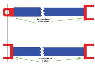
C. Visually inspect driveshaft for proper phasing. (See illustration.)
