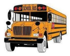
**Type D:** A Type "D" school bus is constructed utilizing a stripped chassis. The entrance door is ahead of the front wheels; also known as *rear or front engine transit style school buses*.
